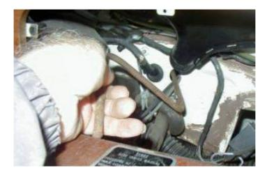
The tool is positioned properly when the middle segment is horizontal and the other two segments are nearly vertical. The vertical segment in the engine compartment should rest against the hood release lever as shown in following photo.
