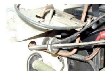
The hood is released by pushing the bottom of the tool to the left causing it to rotate around the middle segment and the top to move to the right and pressing against the hood release lever.
