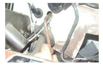
One caution, the positive battery terminal is near the hood release lever. If the rubber insulation is missing from the cable connector, it may be possible to get the tool on the positive terminal. A friend managed to vaporize part of a large screwdriver while attempting to open his hood through this same hole. If you're really concerned about this, you can insulate the end
