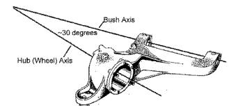
**Bushes:** The standard bushes are made of rubber with metal sleeves in the middle. After years of use, the sleeves tend to migrate to one side of the bush. Since the forces on the inside and on the outside bushes are different,
